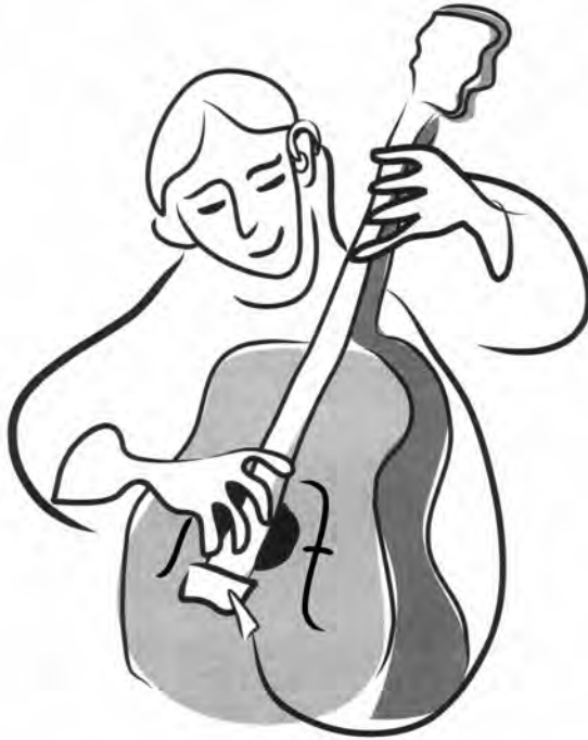
Figure 3-7: An acoustic monitoring device consists of a length of standard hearing aid tubing that joins an earplug (usually a vented/tuned earplug) to a bass instrument. The attachment can be clipped onto the tailpiece, taped to the instrument body, or simply placed in a “f-hole”.
