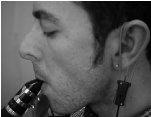
Figure 3-1: Musician being tested with a real-ear measurement system while playing the clarinet. A probe is inserted into the ear canal between the earplug and the ear canal wall while the clarinet is being played.
